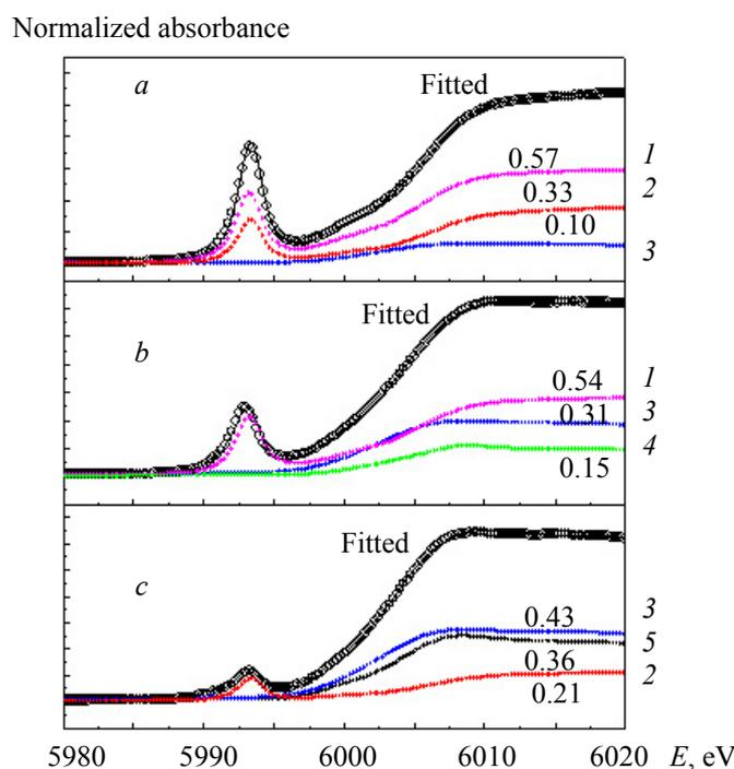
Fig. 1. The least-squares fitted XANES spectra of chromium compounds (Cr(VI)-HA (1),  $\text{Cr(VI)}_{\text{ads}}$  (2), Cr(III)-HA (3), Cr(III) ion (4),  $\text{Cr(III)}_{\text{ads}}$  (5)): (a) adsorbed in ZSM-5, (b) extracted in  $[\text{C}_4\text{mim}]\text{Cl}$ , and (c) remains in ZSM-5 (not extractable).
