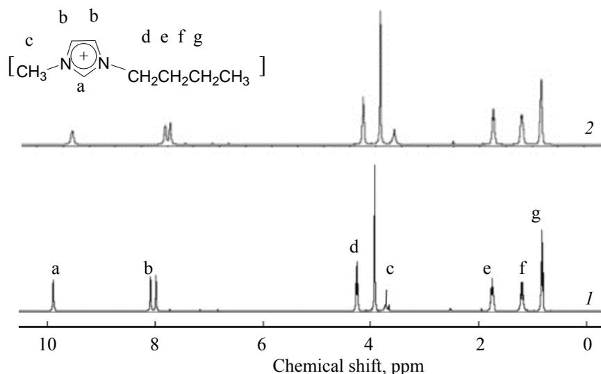
Fig. 2.  $^1\text{H}$  NMR spectra of the IL ( $[\text{C}_4\text{mim}]\text{Cl}$ ) prior to (1) and after (2) extraction.
