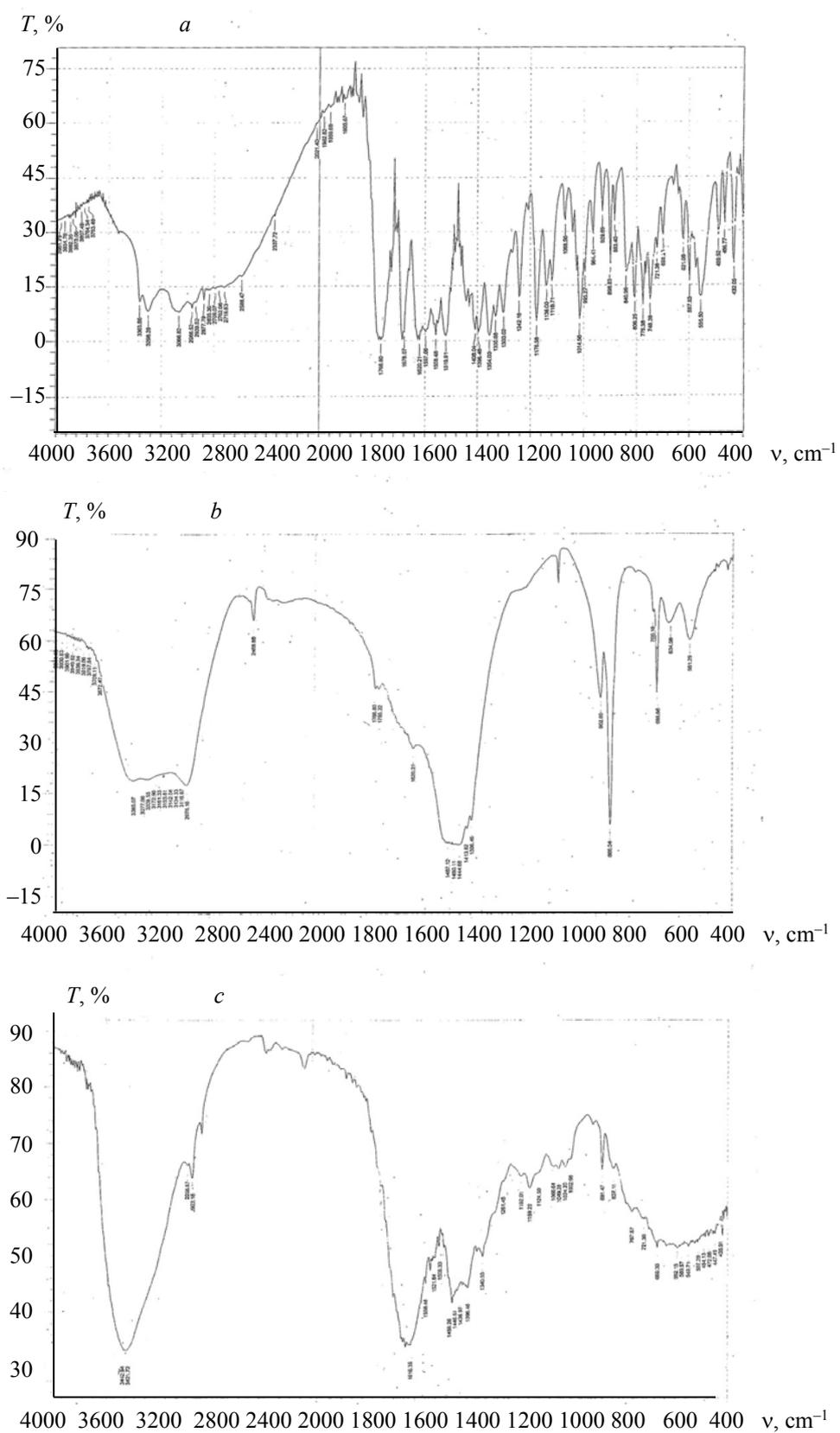
Fig. 1. IR spectrum of a) intact CEF, b) acid-induced degradation product of CEF, and c) alkali-induced degradation product of CEF.
