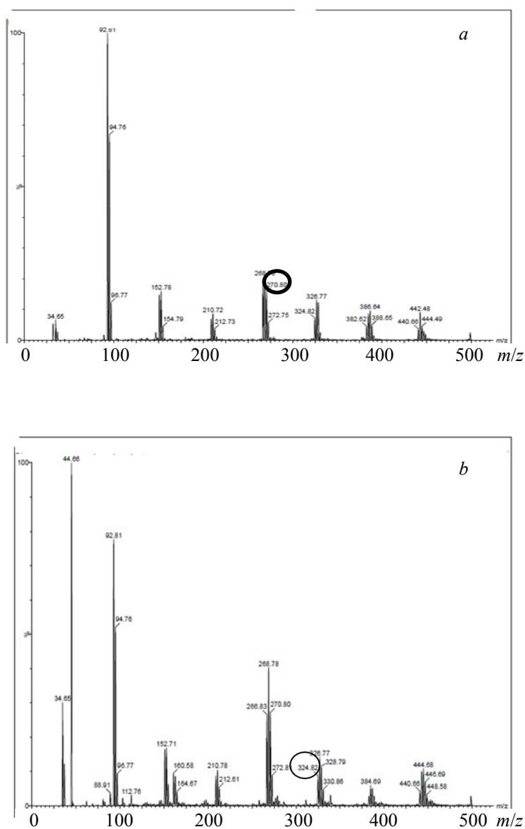
Fig. 2. Mass spectrum of a) acid degradation product of CEF and b) alkali degradation product of CEF.
